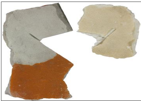
Figure (7) cleaning of naturally stained marble shows a cleaned and an uncleaned area, the piece at the right shows the poultice after removal.
